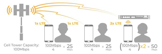
In this example, the third user is using a Pepwave MAX device and has installed an additional LTE data SIM. There are now three devices with four LTE connections connected to the cell tower.
