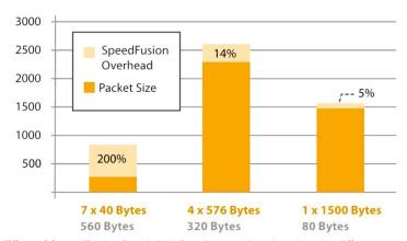
Effect of SpeedFusion Bandwidth Bonding overhead against the different packet sizes and quantities of the IMIX standard
