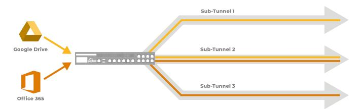
This is achieved through user defined sub-tunnels. Within a SpeedFusion connection, you can define up to five sub-tunnels. Within each sub-tunnel, you can specify which WAN connections to use, set bandwidth limits, as well as configure WAN smoothing and FEC. Once you have defined these tunnels, you can then use outbound policy to steer traffic based on protocol (TCP vs UDP), Port, and Application.
